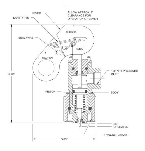
MATERIAL LEVER: STAINLESS STEEL BODY AND PISTON: BRASS
