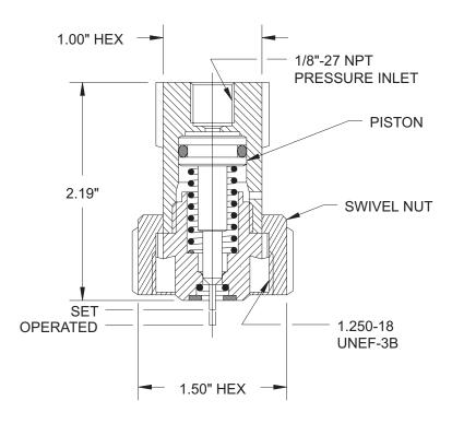
MATERIAL BODY, RETAINING NUT AND PISTON: BRASS
