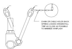
SPRING LOADED LIQUID OR GAS SHUTOFF VALVE
