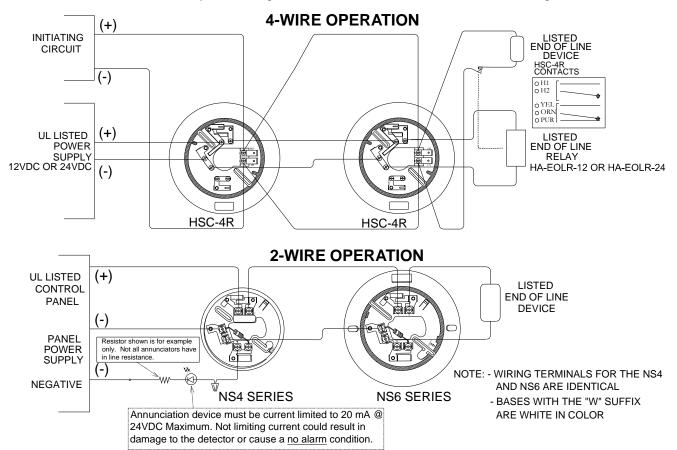
2-wire relay wiring diagram is also available
