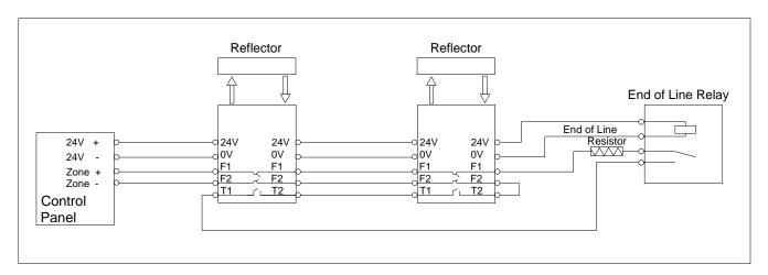
NOTE: End of line relay and trouble contacts are closed when power is applied.
