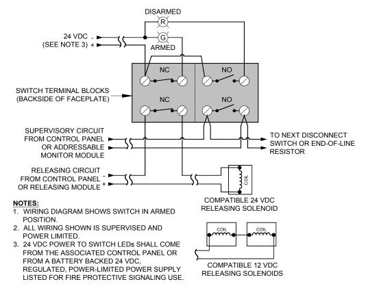
**Exhibit 5: Wiring Diagram of Switch with LEDs**
