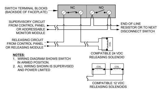
**Exhibit 4: Wiring Diagram of Switch without LEDs**
