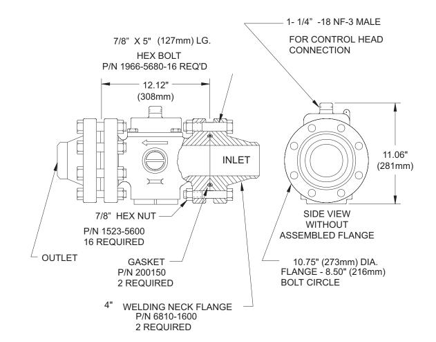
MATERIALS VALVE BODY; BRASS GASKET: IRON FLANGES, BOLTS & NUTS: STEEL
