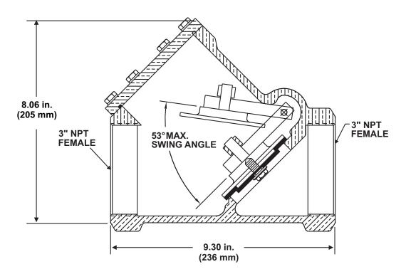
Note: The valve must be installed with the arrow pointing in the direction of flow.
