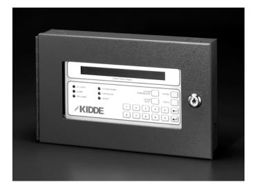
The PEGAsys control panel or one RDCM can be programmed as the master unit to control the system under alarm or fault conditions. Operation of an alternate (non-master) unit will grant this module exclusive control of the system for a period of 30 seconds. To prevent conflicting inputs under these conditions, attempts to input from another module will prompt a lockout-display message on the module attempting the interrupt. Under all conditions, the master will have immediate system control.
