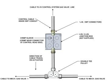
Figure 4. Double Tee Pulley with Two Mechanical Gas Valves (XV Control System only)
