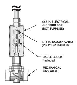
Figure 2. Typical Mechanical Gas Valve Installation
