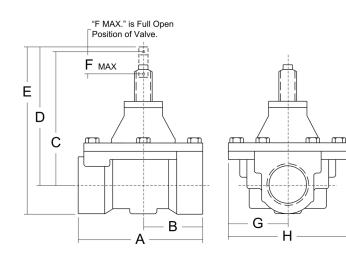
Figure 3. Dimensions of the Mechanical Gas Valve
