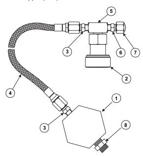
Figure 2. Nitrogen Transfer Components
