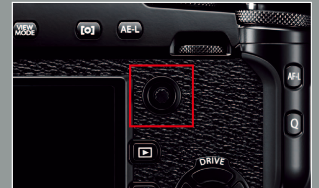
Clicking the focus lever in the centre will instantly return the focus area back to the central point.
