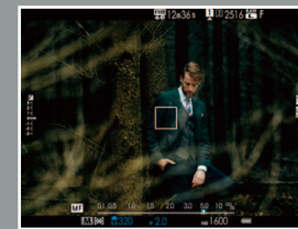
The Depth of Field Scale, displayed as a blue bar in the distance index, gives a visual guide when manually pre-focusing.
