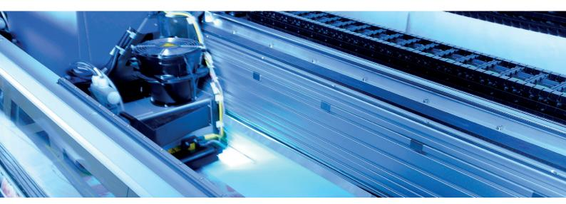
UV curing inkjet is quickly becoming the technology of choice for the production of superwide graphics. It has enabled industrial inkjet to reach new levels of productivity and versatility as UV inkjet is instant curing and the process is clean, efficient and waste is minimised.
