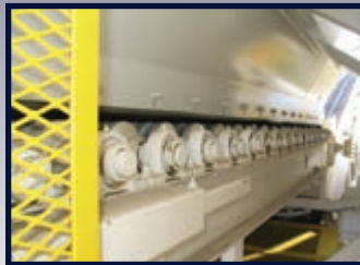
Impact roller assembly c/w 23/8" shafts and bearings
