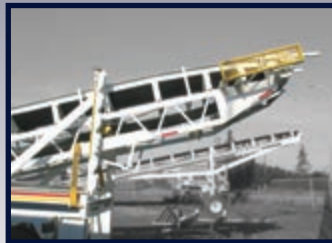
Lattice frame conveyor w/adjustable height spill boards full-length
