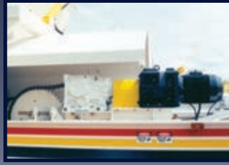
Torspec vari-speed control c/w right angle eurodrive and chain/sprocket final drive
