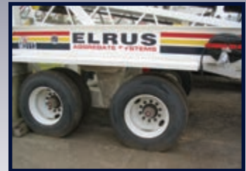
ELRUS HD walking beam suspension
