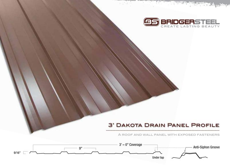
BRIDGER STEEL'S MOST ECONOMICAL INTERIOR/ EXTERIOR PANEL WITH CLEAN LINES, IT CAN BE USED FOR AGRICULTURAL, COMMERCIAL AND RESIDENTIAL APPLICATIONS. FEATURING A 5 DEGREE OVERBEND ON OVERLAP COMBINED WITH AN ANTI-SIPHON GROOVE ON UNDER LAP FOR SUPERIOR WEATHER TIGHTNESS.
