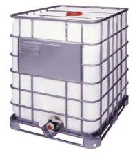
Our Polyethylene Composite IBCs are composed of an inner container extrusion blow-molded from high density polyethylene and an outer container made of rigid welded galvanized tubular steel grid. They work well with steel, wood or plastic pallets.
