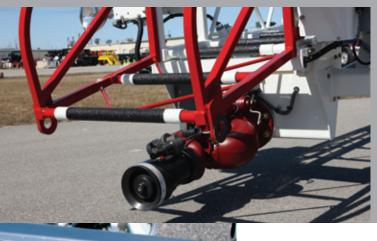
without reducing the rated load capacity. And it can carry that load while flowing 1,500 gpm with a 180° horizontal nozzle sweep at full extension from -8° to +75°.
