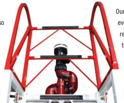
Our egress is easy to replace. If it's ever damaged on a call, you simply replace it with a new one, rather than replacing the entire fly section.
