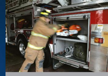
Pierce<sup>®</sup> Bodies feature lateral frame extensions built directly off the chassis frame rails – the strongest part of the truck. That's why we can deliver a 500 lb. compartment floor capacity and a body structure that comes with a 10-year warranty. Maximize every inch of space with our selection of two-way slide-out trays, tilt trays, floor-mounted trays, tool boxes, swing-out toolboards and adjustable partitions.
