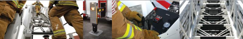
Each ladder is supported by a superior design. One that's fully welded, in compliance with the American Welding Society, by certified welders. Ladder sections are trussed vertically and diagonally and all rungs are welded to each section with k-bracing for rigidity. The ladder device comes with a 20-year warranty against structural failure.
