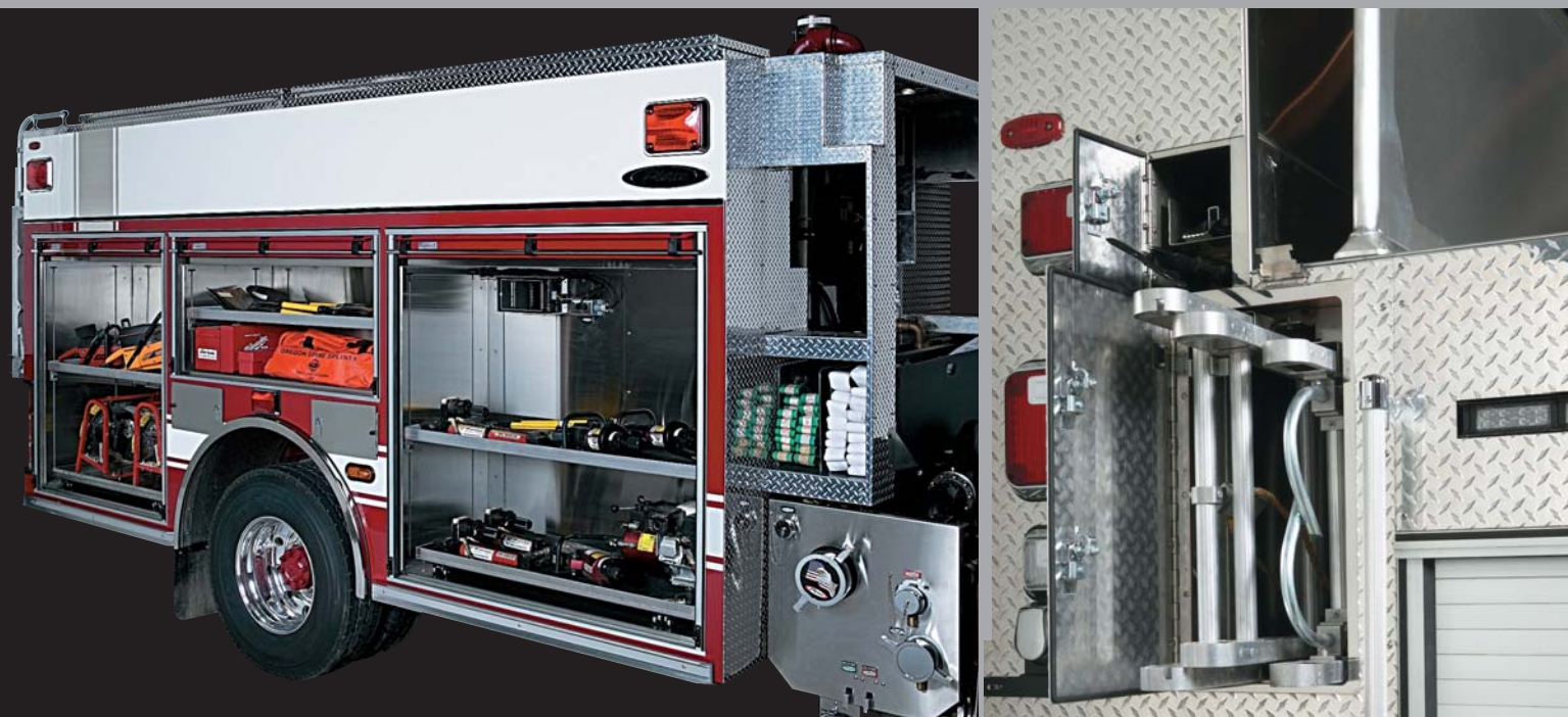
Space-saving rear folding work platform allows for easier access to the hosebed.
