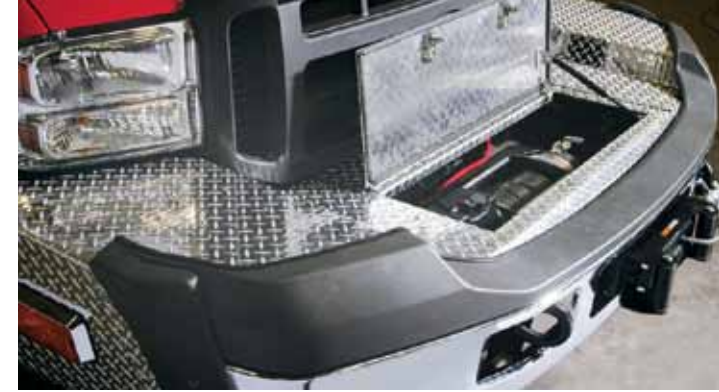
Extended front bumper fitted with optional winch.
