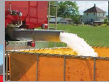
Pierce's exclusive rear 10" tank dump with manual valve and 90-degree directional elbow.
