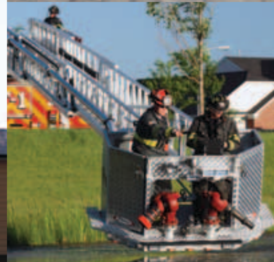
Pierce® aluminum aerials maintain maximum horizontal reach regardless of the degree of angle the platform operates within, anywhere between -11.5 to 76 degrees.
