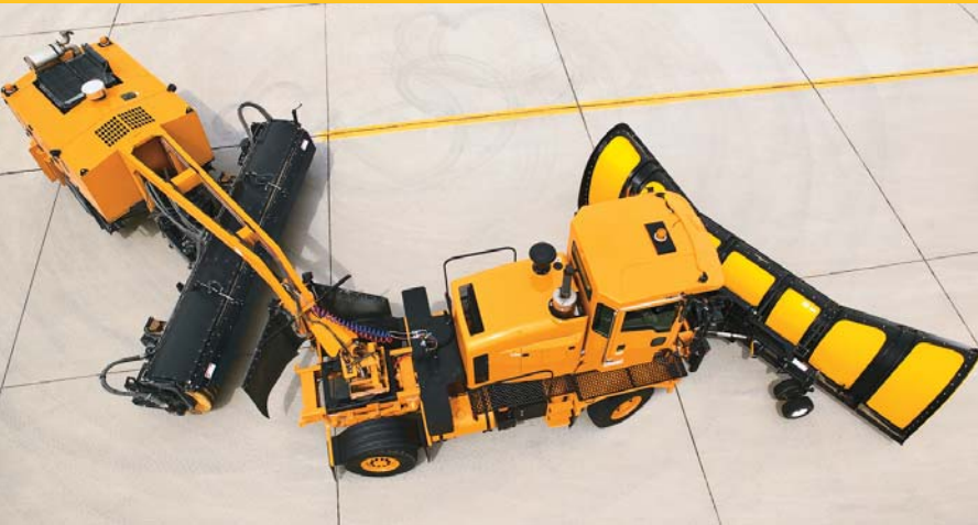
The HT-Series snow tractor with its ALL STEER® electronic all wheel steering system can complete a U-turn in less than 75 feet, wall-to-wall.
