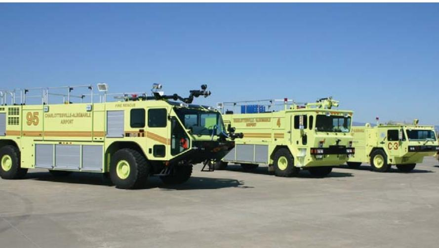
Three generations of ARFF vehicles on display, and on duty: (from left to right) Striker, T-Series and P-19.
