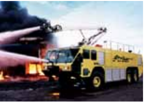
2001 Striker® is introduced, with three models having water capacities of 1500, 3000 and 4500 gallons.
