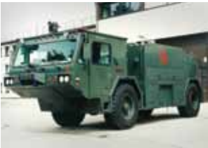
Early 1980’s Production of C-130 air-transportable P-19 for all branches of the military. Vehicle has a water capacity of 1000 gallons.
