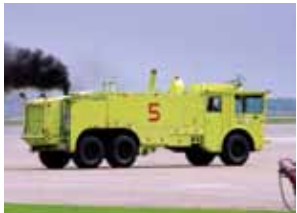
Early 1970’s Company is renamed Oshkosh Truck Corporation. Air Force P-4 airport crash unit is produced, having a water capacity of 1500 gallons.
