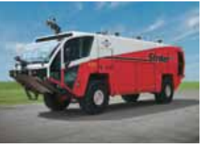
2010: The Striker is redesigned. A new level of versatility provides more storage, lighter body weight, faster acceleration and increased fuel capacity.
