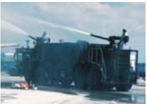
Mid 1970’s P-15 is developed for the Air Force having a water capacity of 6200 gallons.
