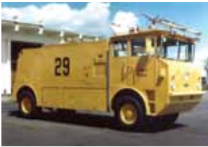
Early 1970’s Navy MB-1, with a water capacity of 1000 gallons.
