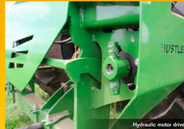
The drive on the cradle is the same at each end
