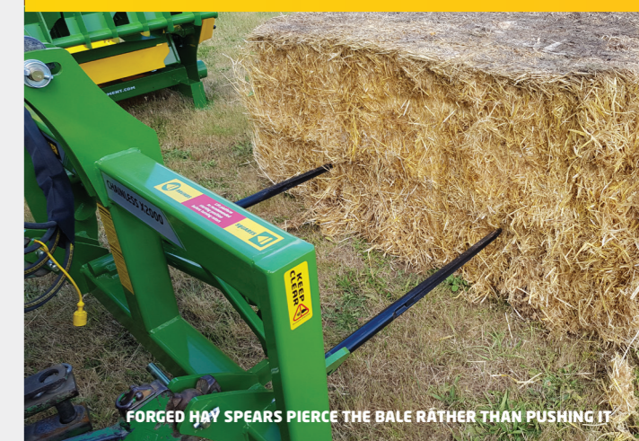
UNEQUAL LENGTH SPEARS MAKE LINING UP EASY WHEN RECONNECTING
