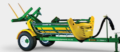
SL700X • Trailed, self-loading • 2 bale capacity • Up to 5 ft wide bales • Total Control Loading
