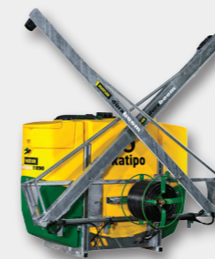
Katipo 890 • Manual controls • 890 litre capacity • 8-12 metre manual fold booms • 50 metre folding hose reel and spray gun
