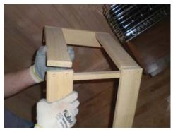
Step 12: Assemble the heater guard with 1-1/2" screws provided according to the pre drilled holes.
