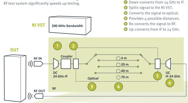
Each DUT is quickly loaded, rotated, and fully tested for its ability to detect stationary and moving objects up to 70 metres away.
