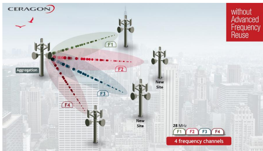
Figure 6: Frequency planning without Advanced Frequency Reuse
