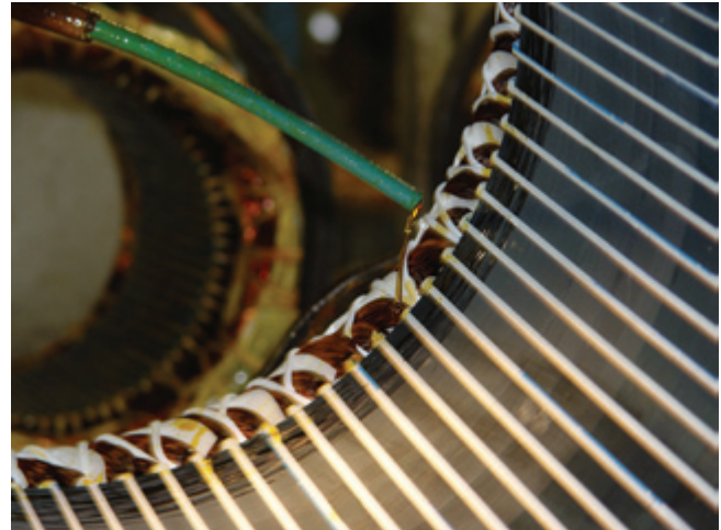
Figure 1.12.c - Resin applied by continuous flow process
