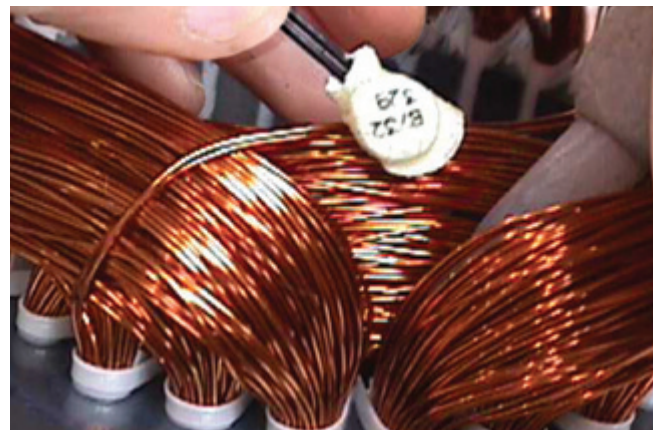
Figure 7.6 - Thermostat installation in the winding
