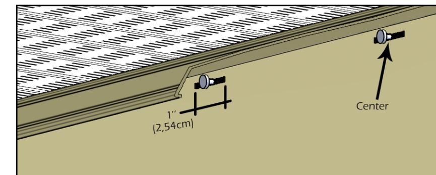
If you need to attach the siding in an area other than the installation hole, create a 1"(2,54 cm) long slot to allow nailing. Always nail in the middle of the slot.
