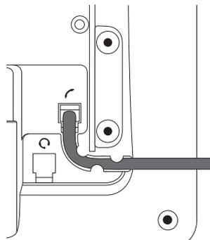
1. Place the top of the grooves on the footstand below the slideguides on the back of the phone.
