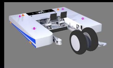
1. Drive the Mototok with opened hydraulical door and lowered platform towards the nose wheel of the aircraft until the nose wheel touches the sliding table. Then press the start-button on the remote control.
