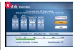
Satellite should be whatever satellite you want to point at. The 72° satellite is recommended as a single satellite solution for DISH HD programming.
