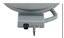
Coax cable connected to main port
