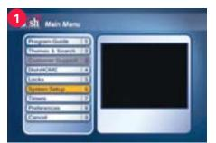
Press Menu on your remote. Select option 6, System Setup. Select option 1, Installation. Select option 1, Point Dish.
