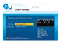
If given the option of selecting a switch type, select Multiswitch. Set the dish type for ROUND 18", Single LNB, or 1 SATELLITE, depending on the wording used in your receiver. Press Continue.
