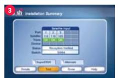
Make sure that there are no checkmarks by SuperDISH or Alternate. Select **Test**.
