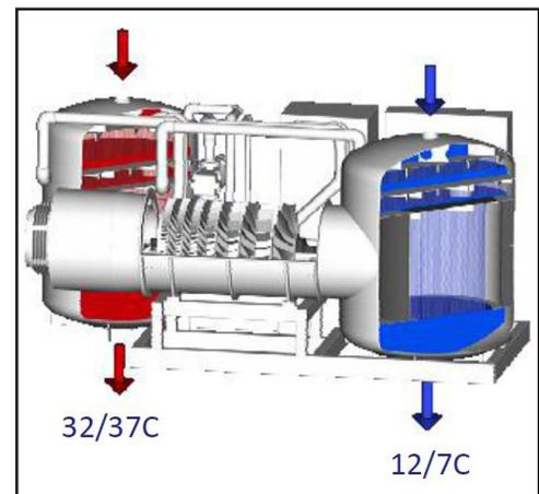
***New type of Axial Compressor with water as refrigerant.***
