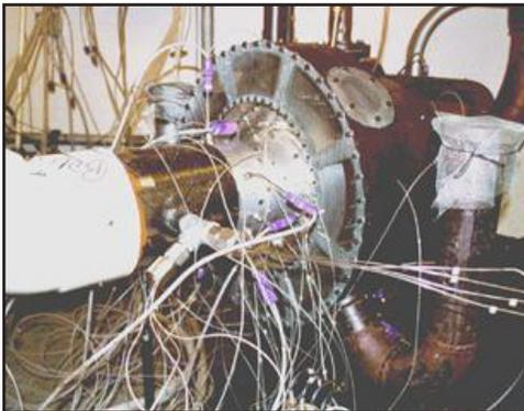
*Axial compressor being tested at low Reynolds number in CN test facility.*
