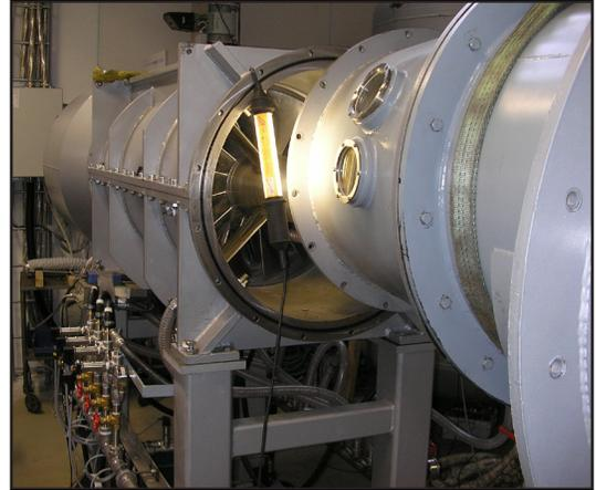
*The smallest compressor has a capacity of 800 kW at 7°C.*
