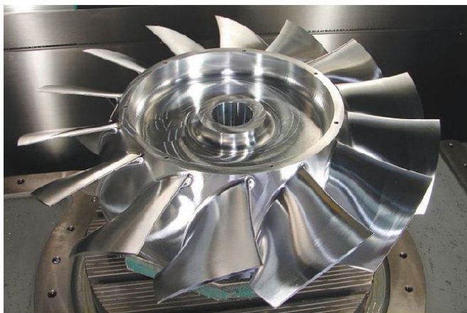
Finished fan with freeform blades. This component did not require an integrated shroud.
