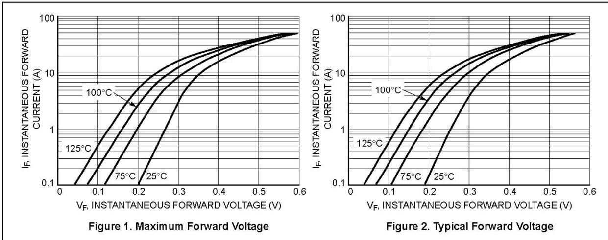
$V_f$  vs.  $I_f$  at various junction temperatures from MBR4015CTL datasheet. This is typical of all three parts.<sup>1</sup>
