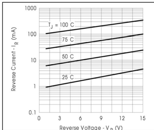
Reverse current vs. reverse voltage at various junction temperatures.<sup>2</sup>
