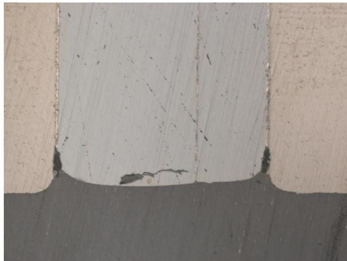
Figure 3: Failed Diode D21 after grinding past the main short
