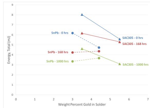
Figure 18: High Speed Shear Test Results, SnPb and SAC305 – Total Energy
