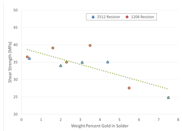
Figure 13: Low Speed Shear Test Results, SAC305 – 1000 hr Aging
