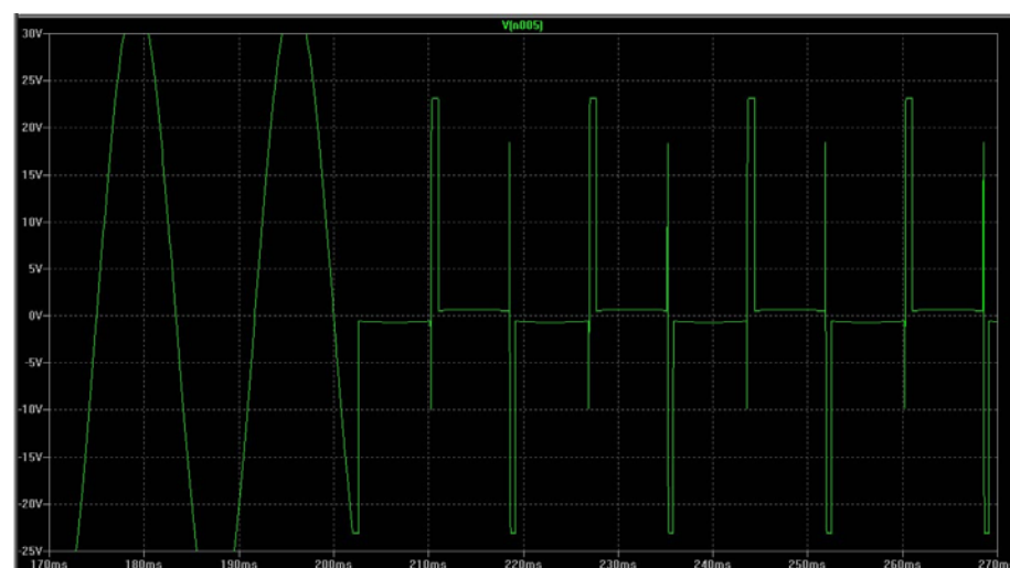
Figure 11 : Variable Triac, Gate Current 16.9mA. Close up of turn-on characteristics
