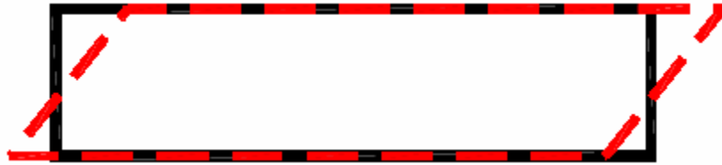
Figure 5: Thickness shear mode of vibration in AT or BT cut crystal 4
