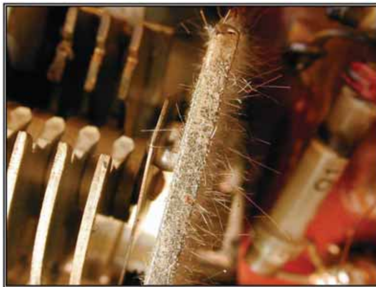
Figure 10: Image of whiskers emanating from a variable air capacitor (manufactured 1959; inspected 2006). The type of tin plating was not identified. Steel plates were typically used in variable air capacitors. Steel substrates are known to greatly increase whisker lengths (Dunn).
