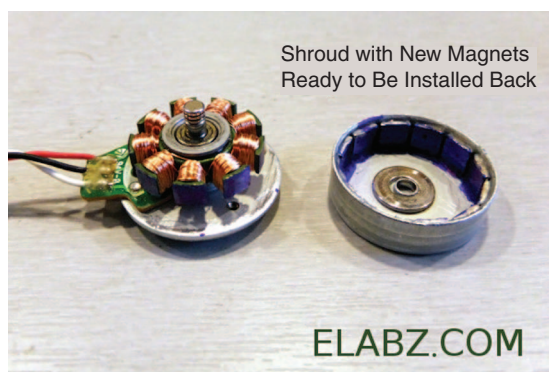
FIGURE 7. The inside of a brushless motor used in an optical drive. (Photo courtesy of Dmitriy Abaimov, http://elabz.com/upgrading-a-dvd-spindle-three-phase-bldc-motor/ .)
