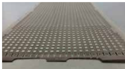
Figure 2: After population, inspection, and finalization on output, a lead frame is placed back into a strip carrier.
