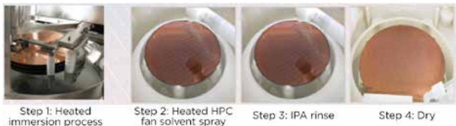
Figure 6: The four-step process flow using a soak-and-spray wet process platform.
