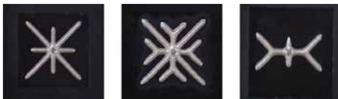
Figure 3: Typical epoxy die attach dispense patterns.
