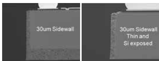
Figure 4: Micrographs of X-section view of eWLCSP™: standard overmolded and thin versions.
