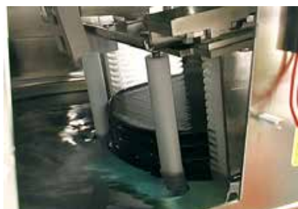
Figure 5: A cassette of wafers soaking in heated solvent.
