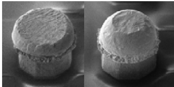
Figure 5: Failed probe mark resulting from high probe force a) post robing b) reflow the same probed bump.
