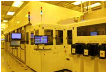
Figure 1: Deca Technologies' wafer-level autoline plating system.
