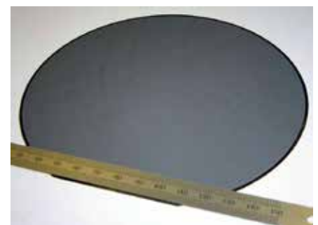
Figure 5: A perimeter ring of uncoated wafer being used in a screen print coating die attach process.
