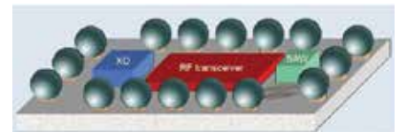
Figure 5: RF module for medical application using IPD/A 2D interposer technology [7-8].
