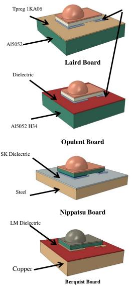
**Figure 3 – Board Configurations**
