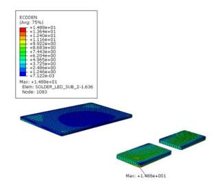
Figure 7 – Strain Energy Density Contour Plot (Cold Dwell)
