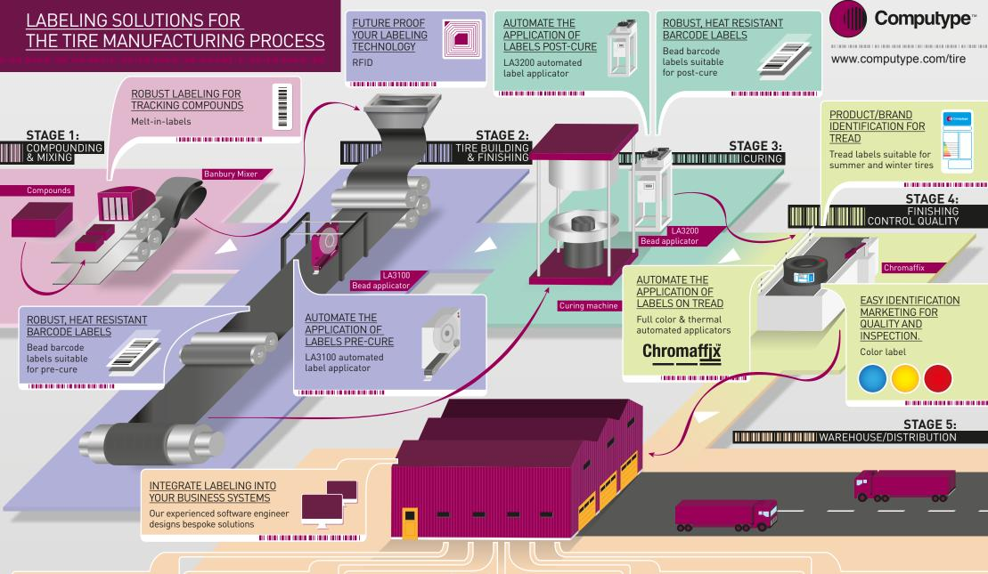
HARDWARE DESIGNED TO INTEGRATE SEAMLESSLY INTO YOUR PRODUCTION LINE
