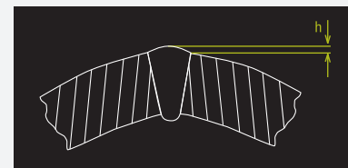
Bead Height Defect
