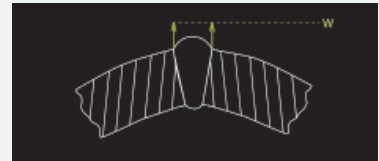
Bead Width Defect
