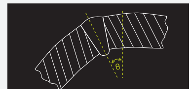
Bead Roll Defect
