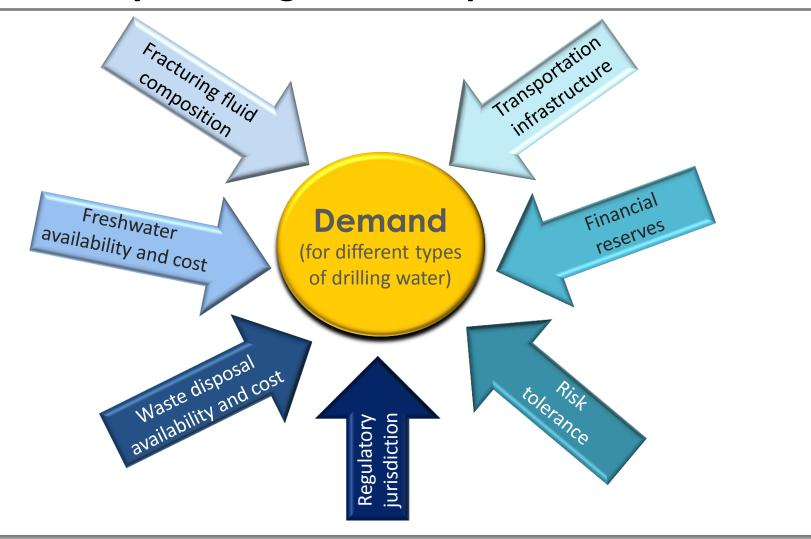
Type of water demanded for recycled water and by-products is complicated by the fluctuation of these critical variables.
