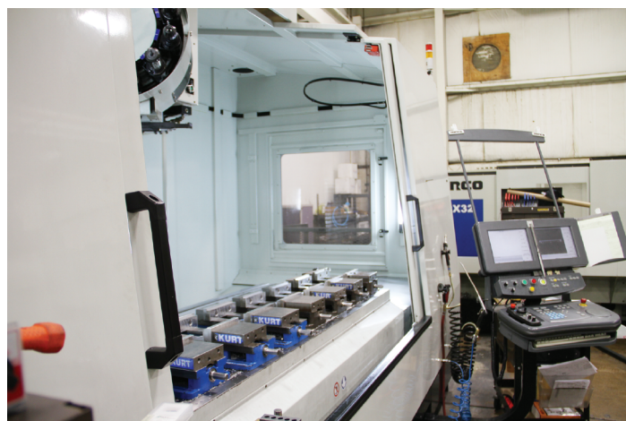
The larger work envelope of the DCX machines supports the large plate work Hallmark does. It is also beneficial for smaller jobs because users can do an entire batch at one time with multiple fixtures on the table.
