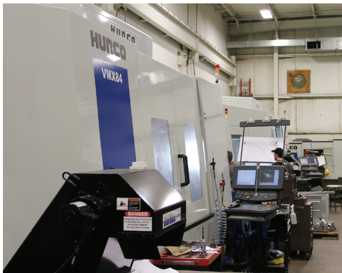
Hurco VMX84 mill. The Hurco was chosen because of its integrated control that includes conversational programming. "The control's operating system is easy to use and it made it easy to train employees who had never programmed a CNC machine before," said George Richards.
